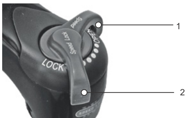
Figure 62: Suntour compression adjuster in open (1) and closed (2) position
