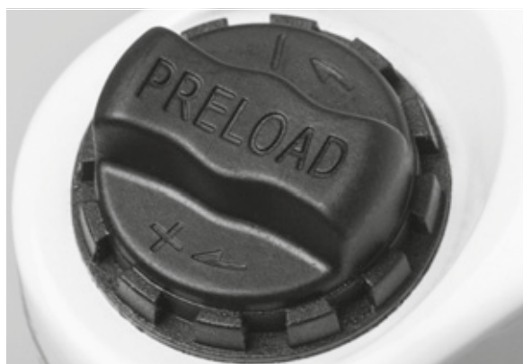
Figure 40: Sag setting wheel on the suspension fork crown
