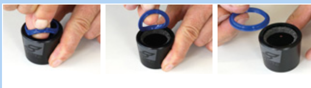
Illustration 240 : Retirer le joint anti-poussière
