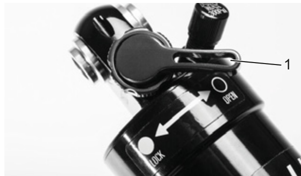
Figure 80: Suntour compression adjuster open (1)
