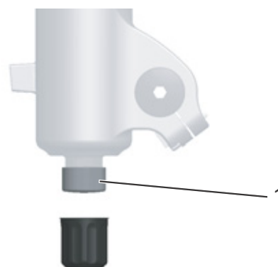
Figure 59: FOX rebound adjuster (1) on the fork
