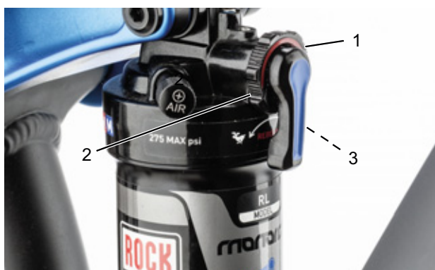
Figure 82: Setting the rebound damper strength on the rear frame damper setting wheel (1)
