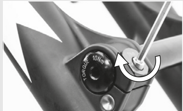
Figure 30: Tightening the axle
